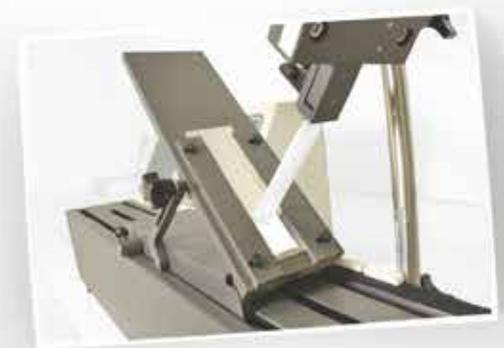
*We follow ASTM International Designation D 3330/D 3330M-04 Method F: Standard Test Method for Peel Adhesion of Pressure-Sensitive Tape as a guideline for our Peel Adhesion test but modify it to include corrugated cardboard.*
